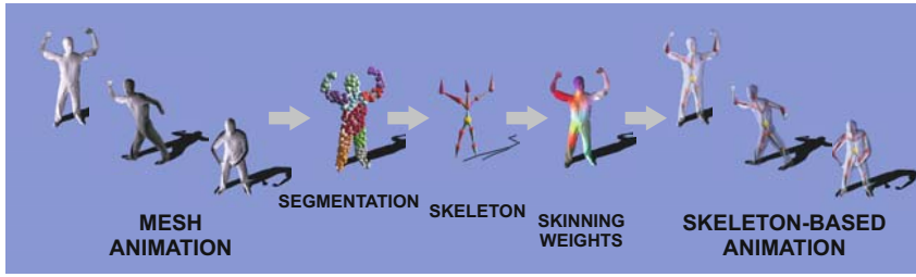
Fig. 14.2 Overview of our algorithm: using an animated mesh as input, our approach segments the model into plausible approximately rigid surface patches, estimates the kinematic skeleton and its motion parameters, and calculates the skinning weights connecting the skeleton to the mesh. The output is a skeleton-based version of the input mesh animation. Reprinted from [2] © Wiley-Blackwell.
